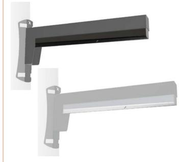
Pole mount, down-firing passive speaker, featuring one horizontal 8  $\times$  2" cone-driver "Pure Array Technology" with protective housing structure and mounting bracket. In the vocal frequency range, the speaker allows a 120° by 15° coverage. High pass filter at 160Hz. IP rating 66. Available in black or white.
