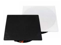
Square speaker for either in-wall or in-ceiling mount, consisting of a 3" coaxial cone and an external 100 V transformer box with 16-8-4-2 W power taps. 130° wide coverage. ABS chassis and stainless steel square protection grille painted in white or black.
