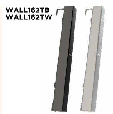
Passive speaker for either wall or ceiling mount including two L brackets, featuring one "Pure Array Technology" of 16x 2" cone drivers and a built-in 100 V transformer with 64-32-16-8 W power taps. In the vocal frequency range, the speaker assures coverage of 120° x 7°. IP rating 65. Available in black or white.
