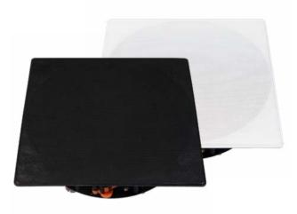
Square speaker for either in-wall or in-ceiling mount, 5,25" coaxial driver 0.75" titanium dome tweeter tiltinge and built-in 100 V transformer with 16-8-4-2 W power taps. 120° wide coverage. ABS chassis and stainless steel round protection grille painted in white or black.
