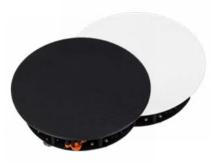
Round speaker for either in-wall or in-ceiling mount, consisting of a 3" coaxial cone and an external 100 V transformer box with 16-8-4-2 W power taps. 130° wide coverage. ABS chassis and stainless steel round protection grille painted in white or black.
