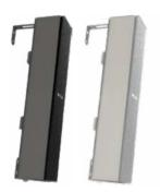
Passive speaker for either wall or ceiling mount including two L brackets, featuring one "Pure Array Technology" of  $4 \times 2$ " cone drivers and a built-in 100 V transformer with 16-8-4-2 W power taps. In the vocal frequency range, the speaker assures coverage of 120° x 25°. IP rating 65. Available in black or white.
