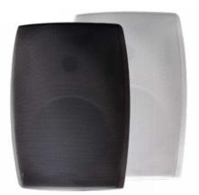
4" full-range, two-way, wall mount, point source speaker, with front protection grille, featuring built-in 100V transformer with 20-10 W power taps. Wall bracket included. Coverage angle 90°. Available in black or white.
